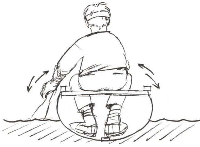
CENTRE OF GRAVITY HIGH. CANOE WANTS TO ROTATE (UPSET).
