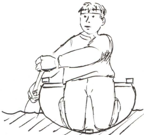
CENTRE OF GRAVITY LOW. CANOE IS STABLE.
